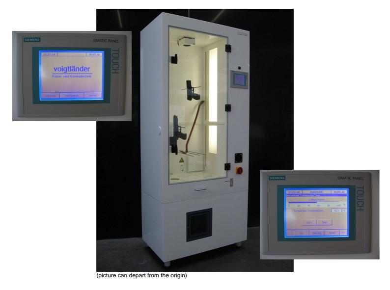
The Cyanoacrylate fuming chamber, now available with touch panel, is a good method to secure evidence for all items with non-absorbent surface.
